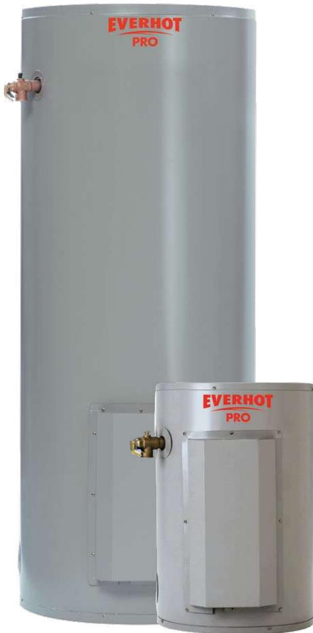
Everhot PRO Heavy Duty Electric is a robust commercial water heater range designed to provide between 240 and 560 litres of hot water in the first hour and 190 to 250L/hr recovery hour after hour at 50°C temperature rise.
