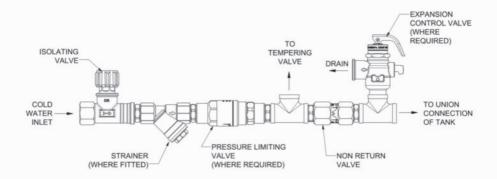
Note: Pressure Limiting Valve required in some locations and recommended where the water saturation index is above +0.40.
